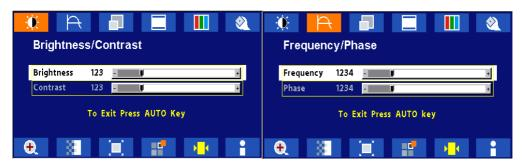
Push "Up" or "Down" button to select between "Brightness" or "Contrast" then push "Select" Use "Left" or "Right" button to adjust Push "Up" or "Down" button to select between "Frequency" or "Phase" then push "Select" Use "Left" or "Right" button to adjust
